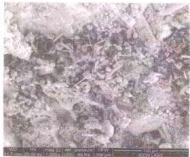
Fig.2 at 100- \mu m Clear Crystals Group was identified With ACI Crystalline Liquid.
